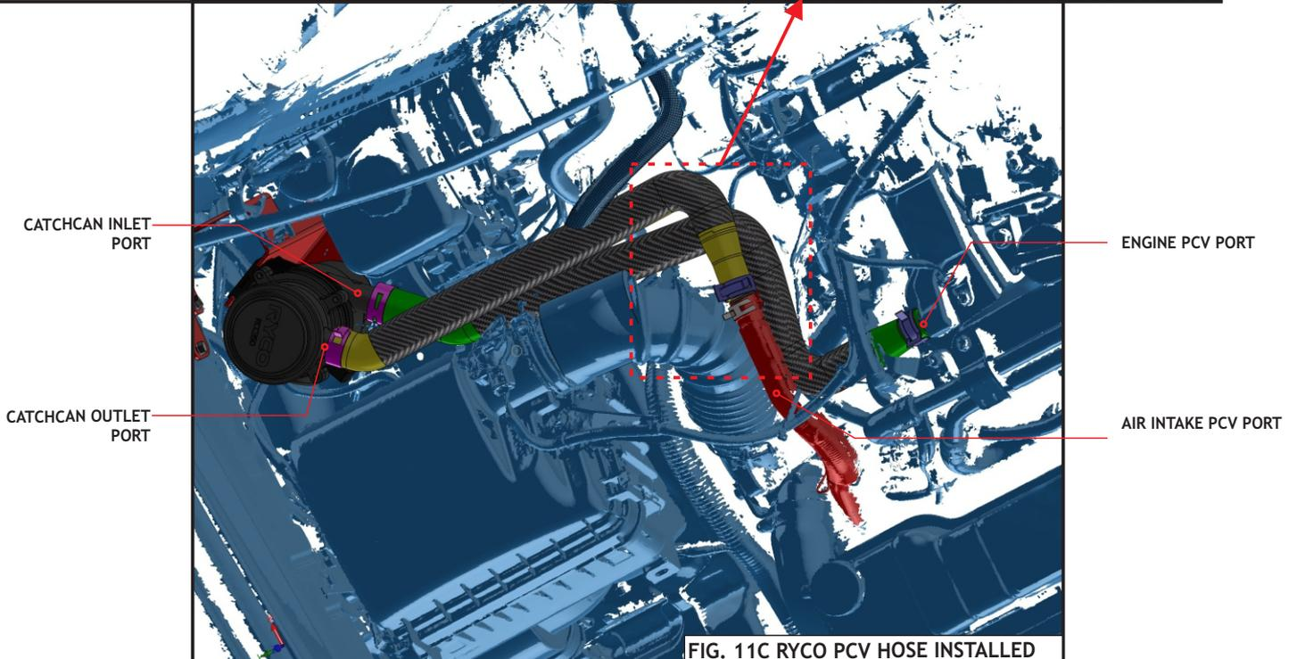
FIG. 11C RYCO PCV HOSE INSTALLED
