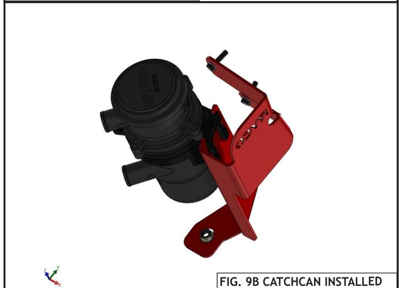
FIG. 9B CATCHCAN INSTALLED
