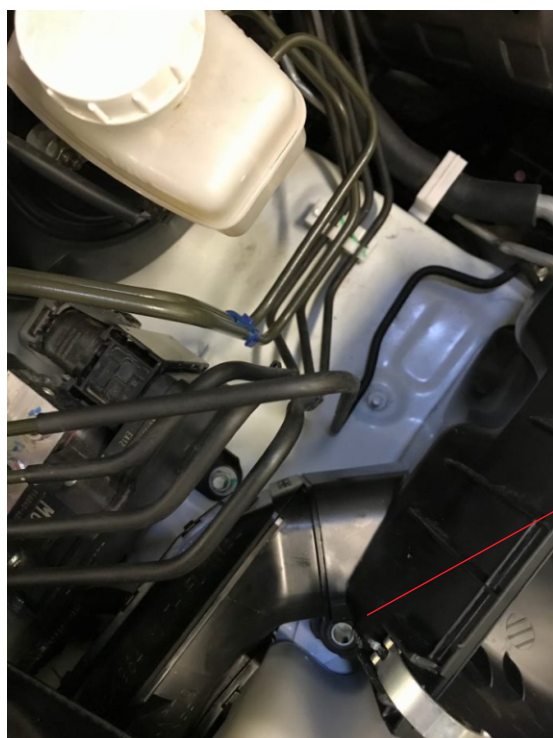
FIG. 8b AIRBOX MOUNTING OEM BOLT/WASHER REMOVAL
