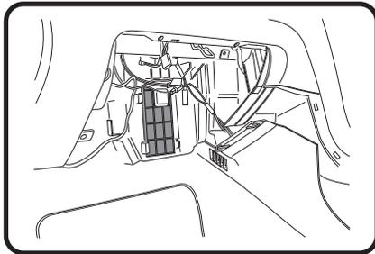
**2:** Remove 5 screws & 2 hex head bolts from around glove box frame, gently pull glove box out until plug for glove box light is visible and disconnect, Remove glove box to expose cover for cabin filter. Remove cover to gain access to filter by pulling out.
