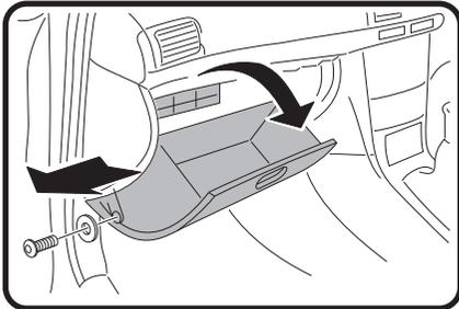
**1: Open glove box, remove screw and washer, then remove the glovebox.**
