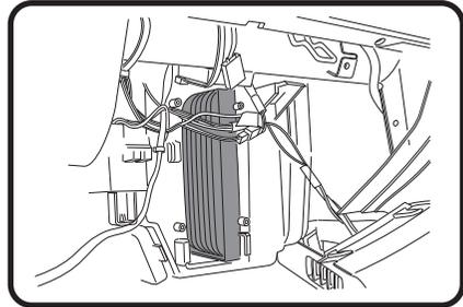
3: Hold wires away from front of housing, Pull used filter out from housing and replace with new RycO RCA104M filter and re-assemble all previously removed components.
