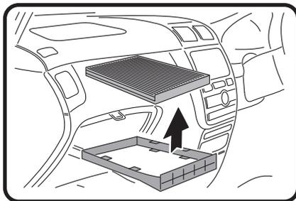
**3:** Remove used filter from tray. Fit new Ryco filter. Refit all previously removed components.
