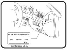
4: Fill in the maintenance label and stick to right hand end of dashboard as shown
