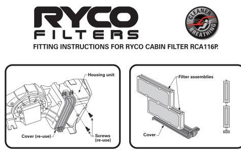
1: Remove cover from housing unit. Remove and discard dirty filters. (do not discard cover or screws.)
