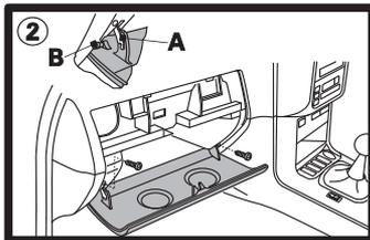
Unclip the retainer for the glove box lid (A), unclip left hand side hinge (B) and lift out the lid, remove 2 screws next to hinges.
