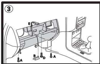
Remove the 2 screws (A) and light (B), pull the plug off the light (C), remove the hex headed bolt (D) and pull out the glove box, pull off the plug (E) on the back of the glove box.
