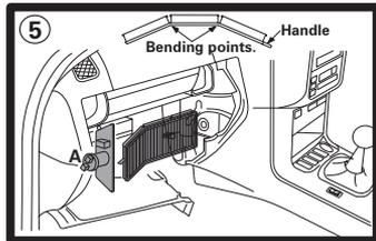
Turn the handle (A) on the duct cover 90°, in an anti-clockwise direction, remove the cover and pull the used filter out by bending at the two folding points, bend the new filter and push into housing with the handle facing outwards.
