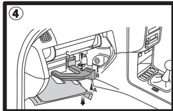
Push the cover down, pull out the 2 plastic pegs (A), pull out the air duct (B) and lift out, move the cable assembly to one side and push the connector block (3) up and out of the holder.
