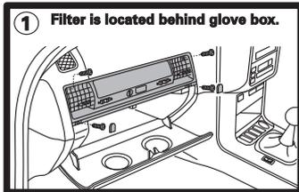
Set ventilator to "0" remove 2 screws, open the glove box, lever out the caps and remove 2 screws from underneath noting their original position, pull out the ventilator panel.
