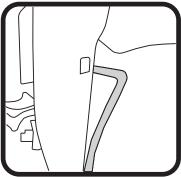
1:Disconnect battery ground lead, wait minimum of 3 minutes to allow the air bag backup system to discharge. Remove the stops at both sides of the glove box.
