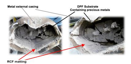
Note: European Environmental Agencies are currently finalising classification and coding of Diesel Particulate Filters containing Refractory Ceramic Fibre (RCF).
