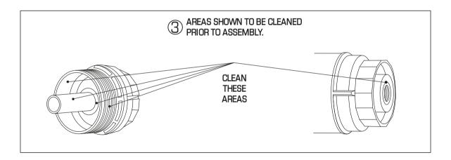
CLEAN MATING THREAD FOR CAP, APPLY COATING OF OIL TO LARGE "O" RING AND FIT IN GROOVE, INSTALL NEW ELEMENT INTO CAP AND SCREW INTO HOUSING BODY, BY HAND THEN TIGHTEN TO 25 ± 5Nm.
