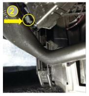
The housing is now visible close to the firewall at the end of the HVAC system. From this point on a small flat srew driver and a 8mm spanner or socket will be required.
