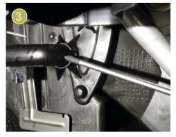
Identify the pipe shown on image 3 and gently pull out to disconnect just the bottom section so it can be moved around to access the bolts securing the servo motor. Unplug the connector of the servo motor shown in image 2.
