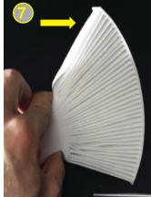
Fit the new filter by squeezing it as shown in image 7. Insert first the top corner of the filter and carefully push inside to avoid damage to the filter. When inserting the filter make sure it is in the right air flow direction. Please refer to the side of the filter for reference. Refit all components in reverse order.
