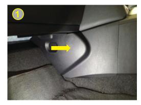
The cabin air filter is located behind the lower trim as indicated in image 1. Pull the trim out slowly starting from the end close to the firewall.
