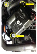
Mo ards the front of the vehicle so the two bolts shown are accessible. Remove and gently pull the servo motor out. Unclip the filter housing clip starting where instructed in image 5 and slide down. The filter will be visble at this point. With a small flat head screw driver or hook, reach for the filter and pull out. It will have to be squeezed in the middle to come out easily. Clean the area from any accumulated debris.
