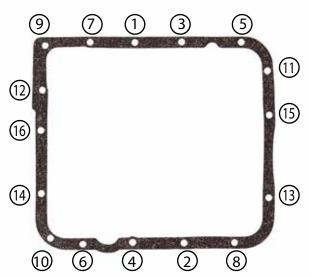
Example of tightening torque sequence
