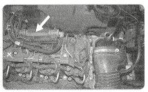
9: Pump the fuel with manual pump until resistance is felt.
