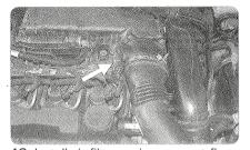
10: Install air filter casing, connect flow meter, start engine, check system for leakage.
